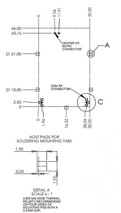
Figure 4 Enabler II-G Host Board Layout
